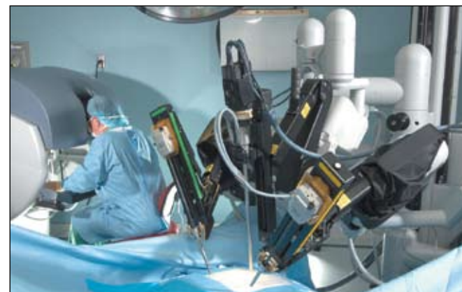
In the da Vinci system, the surgeon sits at a console a few feet from the patient. The device itself is positioned above the patient.
